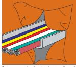
Cut a cross in the barrier to allow the service through
