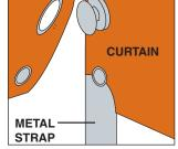
On closing edges of the frame side, rivet one section of steel strap and fix the special turn-button fixings as shown above
