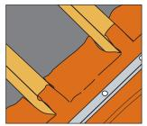
When the barrier overlaps felt battens, it is important to cut the barrier as shown above, tucking it between the battens
