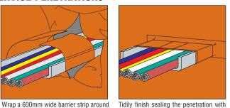
Tidily finish sealing the penetration with Envirograf® adhesive and tape as shown above
