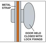
With the door section fixing rings fitted, the door shuts and is locked by turning the turn-button fixings
