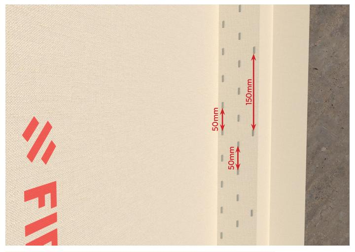
Stapling off the Butt joint is the most labour intensive part of the installation, the speed of which can be vastly improved with the use of a FIREFLY® B16 Stapler or a FIREFLY® FF Pneumatic Staple Gun.
