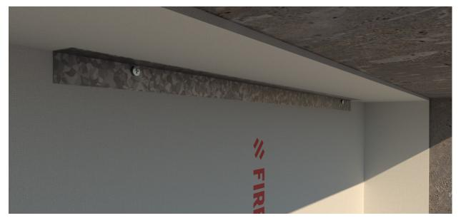
Alternatively the barrier can be clamped in place with a FIREFLY<sup>®</sup> 25 x 25 x 0.7mm Clamping angle. Fixed with FIREFLY<sup>®</sup> Panhead Tek Screws as required. This will typically be easier for a two man installation team.
