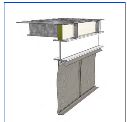
FD090 head detail to intumescently protected structural steel
