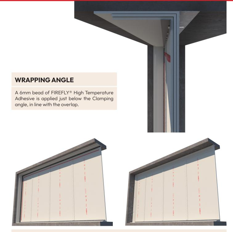
The overlap is brought down and bonded to the bead of FIREFLY® high temperature adhesive, securing the overlap to the body of the barrier.
