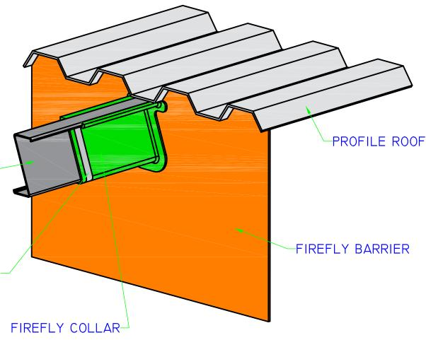
GALVANISED STRAP 25MM X 0.5MM FIXING COLLAR TO PURLIN WITH SUITABLE FIRE RATED FASTENERS-
